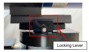
The locking levers on an HAE16C mount are ratchet ones. Pull the lever handle and turn it to the position that the lever is parallel to the saddle or points towards the scope to prevent it interfering with the DEC unit during mount GOTO and tracking.
