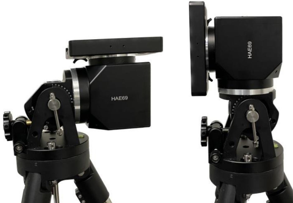
Figure 14. An HAE69 mount set for equator ( 0^{\circ} , left) and altazimuth ( 90^{\circ} , right)
