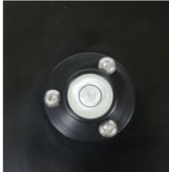
Figure 18. Bubble level for AA mount leveling
