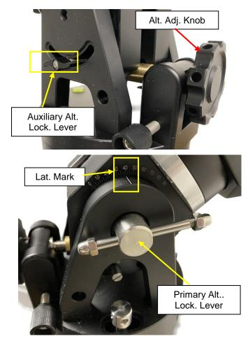
Use the Altitude Adjustment Knob to move the mount to the desired latitude by aligning the scale to the Latitude Mark Line. Tighten both Primary and Auxiliary Locking Lever.
