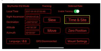
Click on *Time & Site*, then pap on *Sync Current Device Time to Mount* and *Sync Current Device Location to Mount*. to set the mount Time and Site info.
