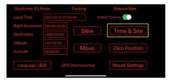
Click on *Time & Site*, then pap on *Sync Current Device Time to Mount* and *Sync Current Device Location to Mount*. to set the mount Time and Site info.
