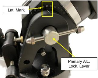
Use the Altitude Adjustment Knob to move the mount to the desired latitude by aligning the scale to the Latitude Mark Line. Tighten both Primary and Auxiliary Locking Lever.
