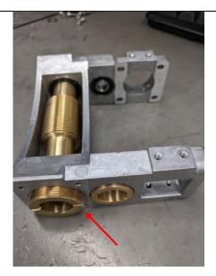
25. Adjust the brown end cap to make sure if RA worm can be rotated freely without any free play. Then fasten the setting screw
