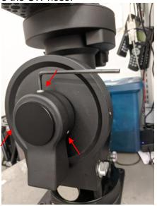
3. Remove four screws (two on left side and two on right side) and then remove the front cover.
