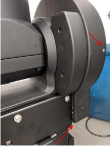
4. Take the mount upside down and loose two locking screws(one on left side and another on right side), and then take the mount base out off the frame and put the base on a box or other object with an appropriate height nearby. Please pay more attention the connection wires between the base and the mount frame.
