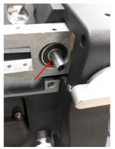
42. Install the brown end cap and tighten it. Push the axle to an appropriate position.
