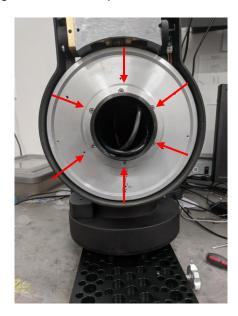
19. Pull out the whole RA worm assembly with belt.
