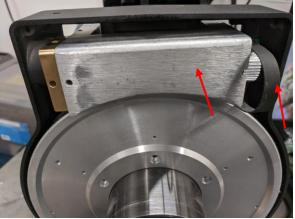
20. Remove four screws and remove the brown support part. Please mark its orientation before remove it
