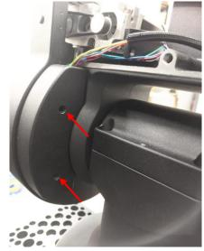
Remove the RA module which RA board is inside. Disconnect two connection wire bundles. (One is to motor and another is to main board)
