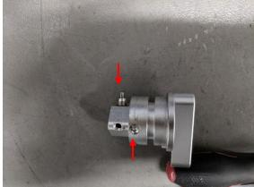
33. Push gear switch knob before the metal post comes out to stops it to be pushed any further. Pay more attention to the small ball.
