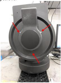
38. Insert a brown washer between mount frame and a bearing inside RA worm housing frame (left side) and make sure it align with each other.
