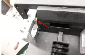
39. Install the axle into the bearing and push it to an appropriate position.
