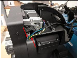
6. Remove three screws on the other side and take off another panel with scale.
