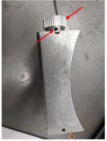
27. Install the encoder wheel. Please do not forget its washer.
