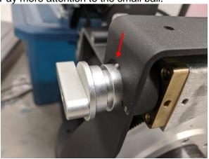
34. Use a flat screw driver to push the metal post down and carefully push the gear switch knob further while moving RA worm assembly up and down slowly if necessary.
