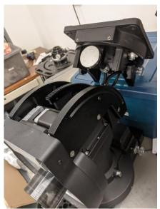
5. Remove four screws and take off the panel and pay more attention to the connection wire arrangement. All of them should be put in a notch in the other side of the panel when assembling later.
