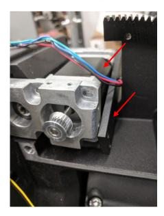
12. Loose three setting screws. Remove the latch for RA gear switch knob.
