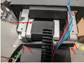
45. To make the belt tight, use a small flat screwdriver to lift the motor a little bit while fastening four screws.
