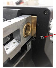
37. Install CW nose by installing one screw and two setting screws.
