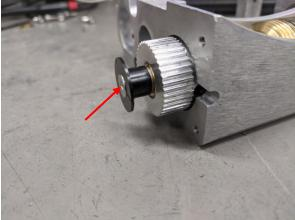
22. Loose two setting screws and remove the pulley.
