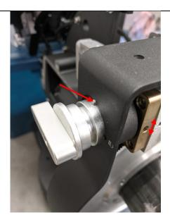
18. Remove six screws and pull out RA ring gear until it does not block RA worm assembly to be pulled out. Please mark the orientation of the RA ring gear first before pull it out.
