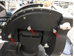
47. Put back another panel while pay more attention to arrange the connection wires well. The two sets of connection wires must be put in the notch which is in the other side of the panel.
