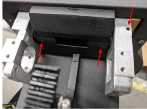
44. Put back RA motor and its protection bar. Install the protection bar by installing four screws.
