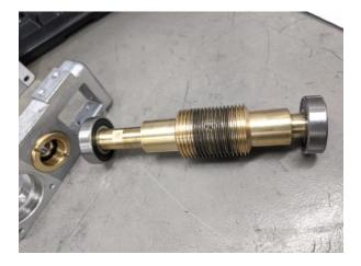
24. Check two bearings and put new worm into RA worm housing. Then install the brown end cap.
