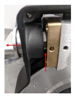
17. Use a flat screw driver to push the metal post down and carefully pull out the gear switch knob further. Please pay more attention to the small ball while pulling out the gear switch knob. If necessary, move RA worm assembly up and down slowly while pulling out the gear switch knob further.
