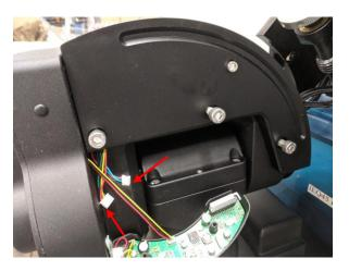
48. Hold and push hard the panel while making sure if the two sets of connection wires can move freely inside and outside of the panel. If any of connection wires cannot move freely, please go to Step 47 and rearrange connection wires and put them all in the notch. At last, connect two connection wire bundles to RA board. (One is to motor and another is to main board)
