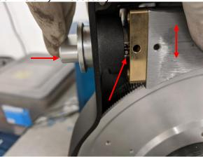
35. Install front cover by installing four screws(one on left, one on right and two on rear)
