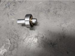
41. Make the worm housing frame (right side) align with mount frame. Then insert the axle with bearing and washer into the hole and the hole in mount frame..
