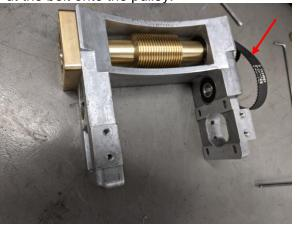
30. Insert the whole RA worm assembly with the belt into the mount frame
