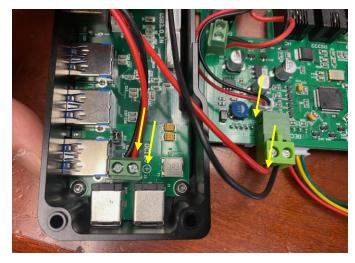
10. After plug all the wires into the socket, put the dovetail saddle back in position first. Then connect the CMS input.
