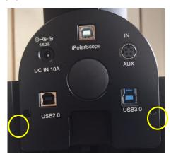
2. Pull the panel open. Disconnect the cables. Remove 3 screws with a 2mm wrench.
